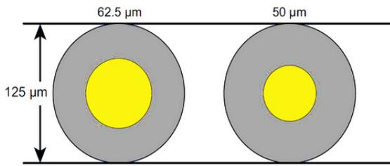
Typical multimode fibre core diameters are 62.5μm (OM1) and 50μm (OM2/OM3/OM4). However, in long cable runs, for example, long distance greater than 3000 feet or 914.4 meters, multiple paths of light can cause signal distortion at the receiving end, resulting in an unclear and incomplete data transmission so designers now call for singlemode fibre in new applications using Gigabit and beyond.
