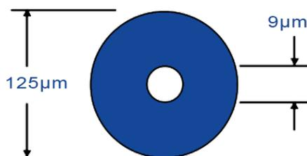
Singlemode fibre generally comes with a relatively narrow diameter, through which only one mode will
